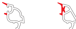
Glassbead 22 mm S-507.06 Glassbead 24 mm S-563.07 0.19 kg/m; Soft PVC 12.8 g/m 0.17 kg/m; Soft PCE 38 g/m
